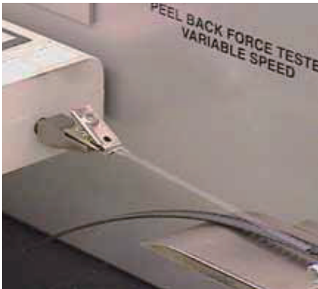
Removal force testing of 3M Universal Cover Tape (UCT) 2688A
