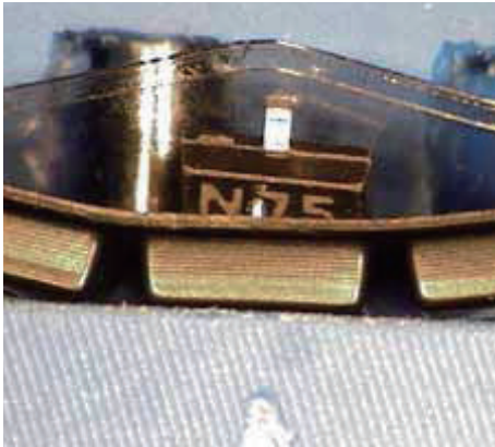
Rework (at peel enabling feature) on 3M™ Universal Cover Tape (UCT) 2688A
